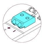
At the output there is a 3-pole WAGO terminal, to which the LED modules are connected.
