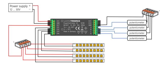
The brightness of the LED modules can be adjusted from O-100% using the assigned potentiometer.
