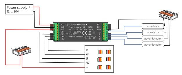
The RGBW LED module can be turned on and off by briefly pressing the switch on input A. By pressing the switch on input B for a longer time, a colour change can be generated where the RGBW LED module cycles through all light colours as long as the switch is actuated.
