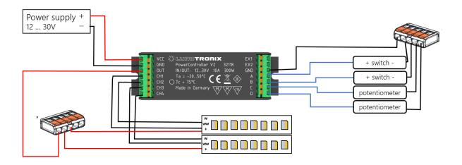
The LED modules can be turned on and off by briefly pressing the switches on input A or B. When held down for a longer time, the tunable white LED modules will be dimmed. Using the potentiometers on C and D, the colour temperature of the LED modules can be changed from warm white to cold white or the other way round.
