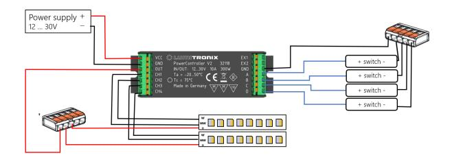
The LED modules can be turned on and off by briefly pressing the switches on input A or B. When held down for a longer time, the tunable white LED modules will be dimmed.
